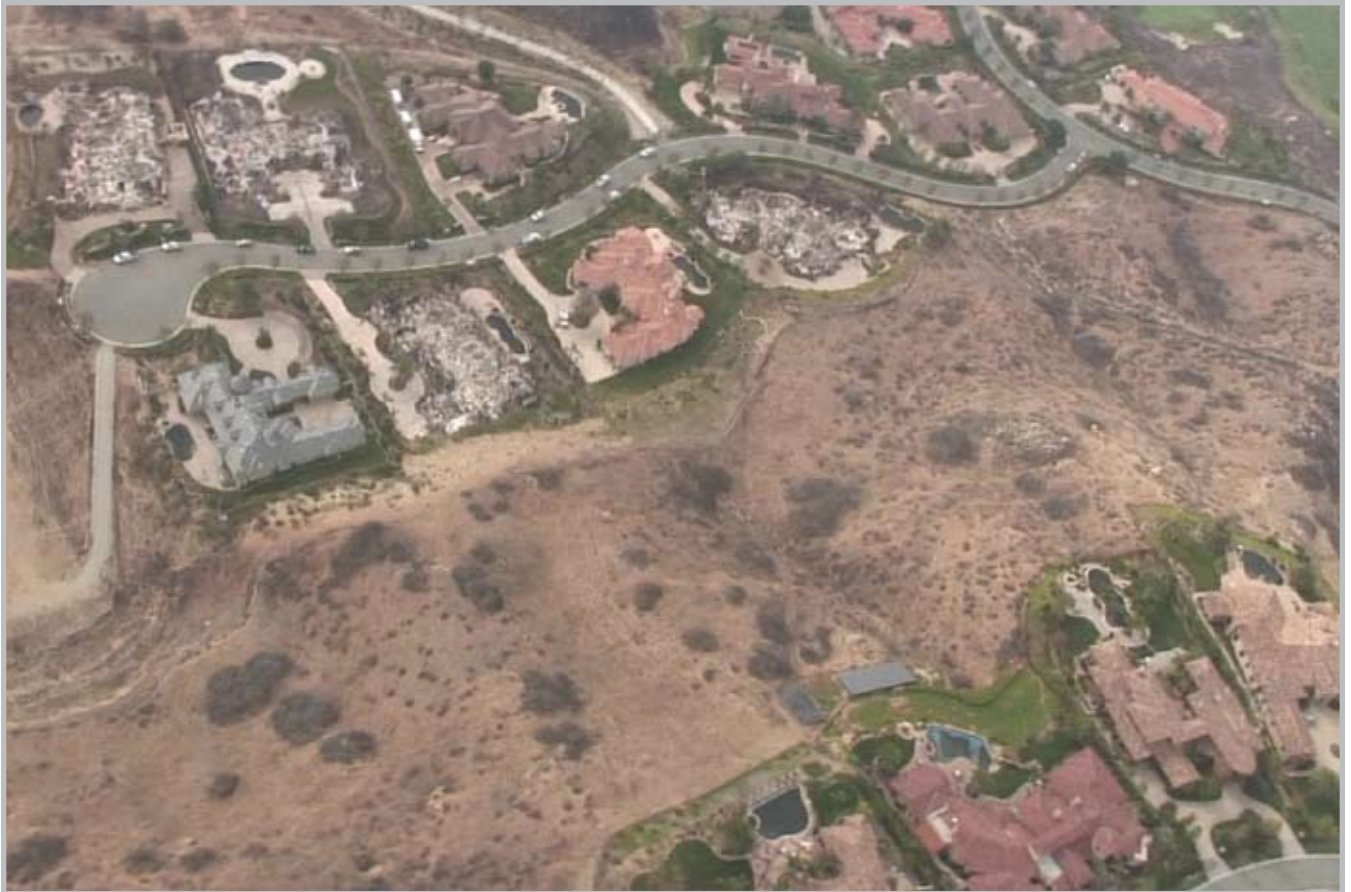
The burnt wildland-urban interface following the Witch Fire in San Diego County, illustrating the low correlation of loss among residential structures (Source: ImageCat)
