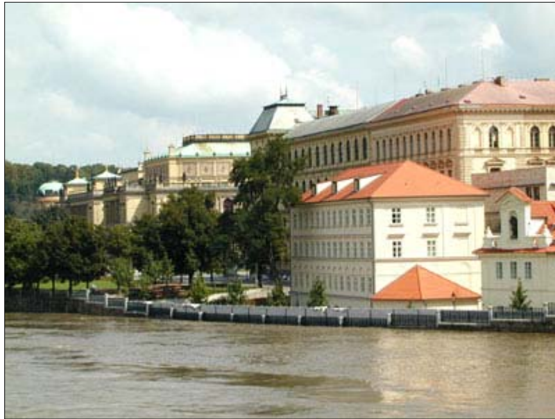
Figure 11. View toward the Old Town showing the temporary flood barrier in front of The Four Seasons Hotel
