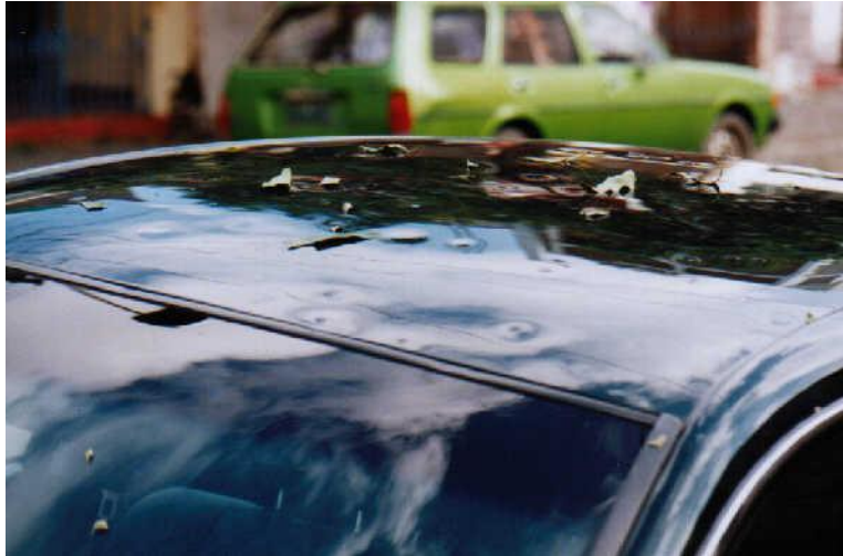
Figure 7: Damage to a car roof as a result of the 1999 Sydney Hailstorm (Source: http://ozthunder.com/chase/chase13.htm )
