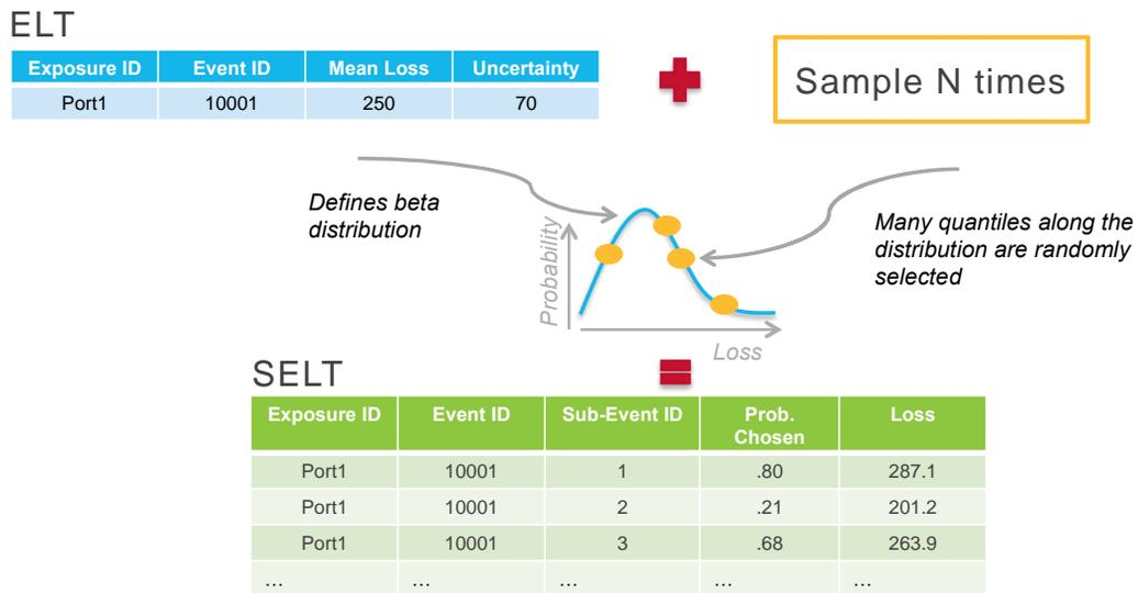
Figure 2: Several points are sampled from the ground-up event loss distribution to generate the SELT.
