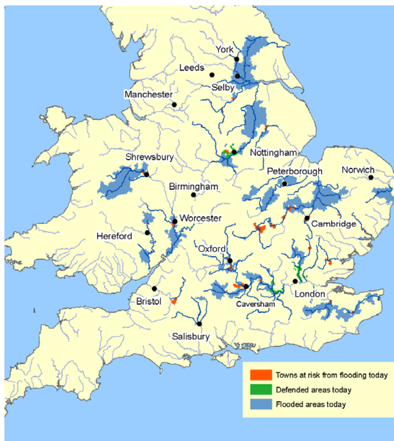
Figure 6: Reconstruction of the 1947 flood footprint, where blue areas indicate postcode sectors where there is significant river flooding in 2007, green areas indicate sectors that flooded in 1947 but would not in 2007 due to flood defenses, and orange areas indicate sectors which could flood in 2007 given the uncertainty in flood defenses for these regions
