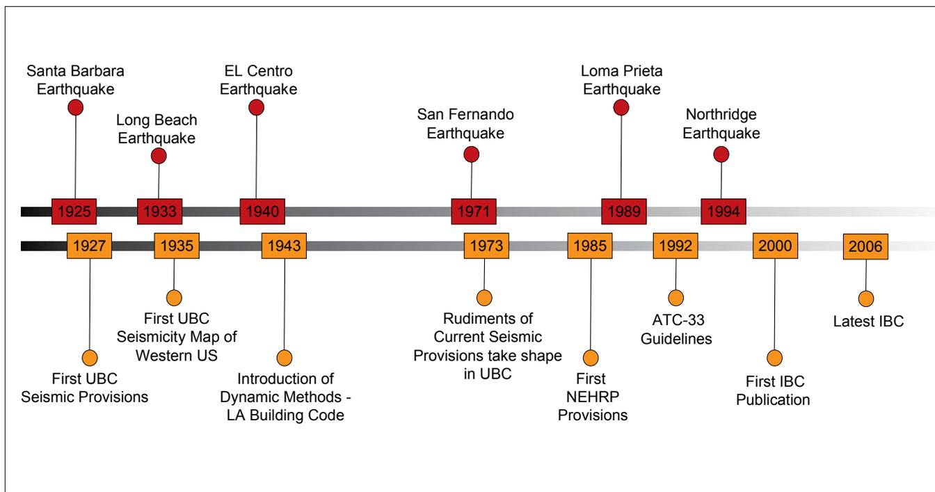
Progression of seismic design provisions in building codes following significant California earthquakes since 1925 (based on *Financial Management of Earthquake Risk, Earthquake Engineering Research Institute, 2000*)
